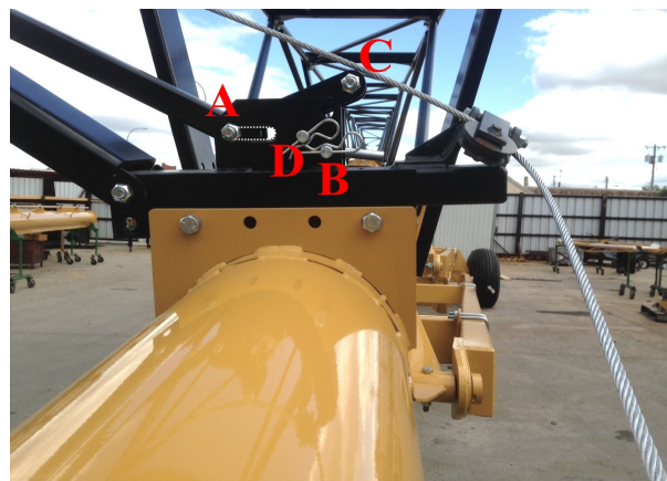
Fig. 8 LIFT ARM OPERATION - HOPPER LOWERED – ARM UNLOCKED
