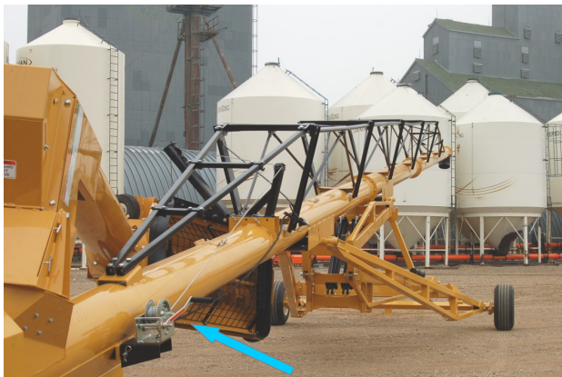
Fig. 5 ALIGN AUGER WHILE IN LOWERED POSTION
