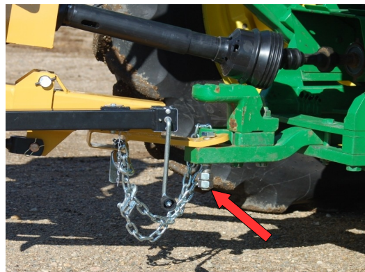
Fig. 4a USE BOLT AS HITCH PIN
