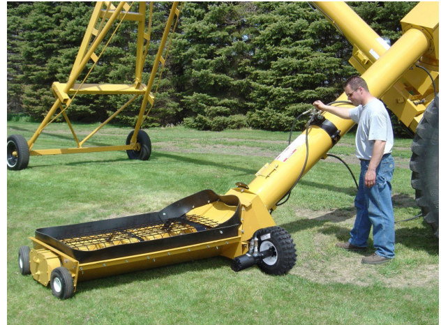
Fig. 12c Power Wheel Option, Hydraulic Double or Single
