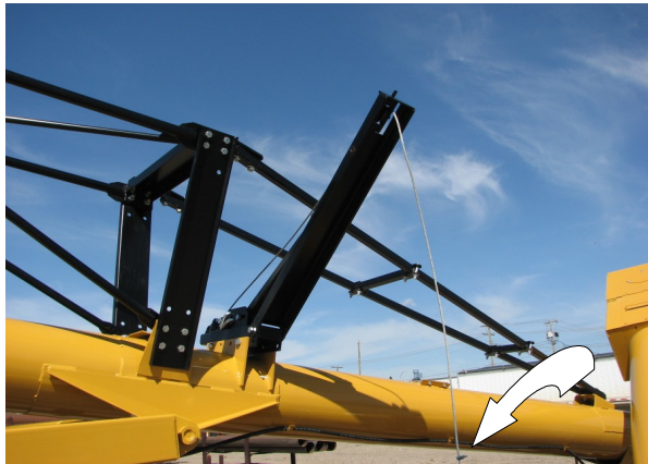
Fig. 15 CABLE CLAMP (ARROW), CURRENT LIFT ARM MECHANISM
