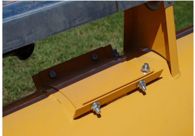
Fig. 33 BEARING REPLACEMENT (Access Covers)
