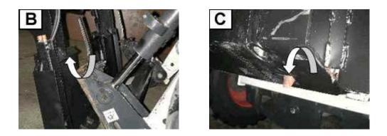
Tilt the skid steer mounting plate backward until the Tele-Boom is slightly off the ground.
